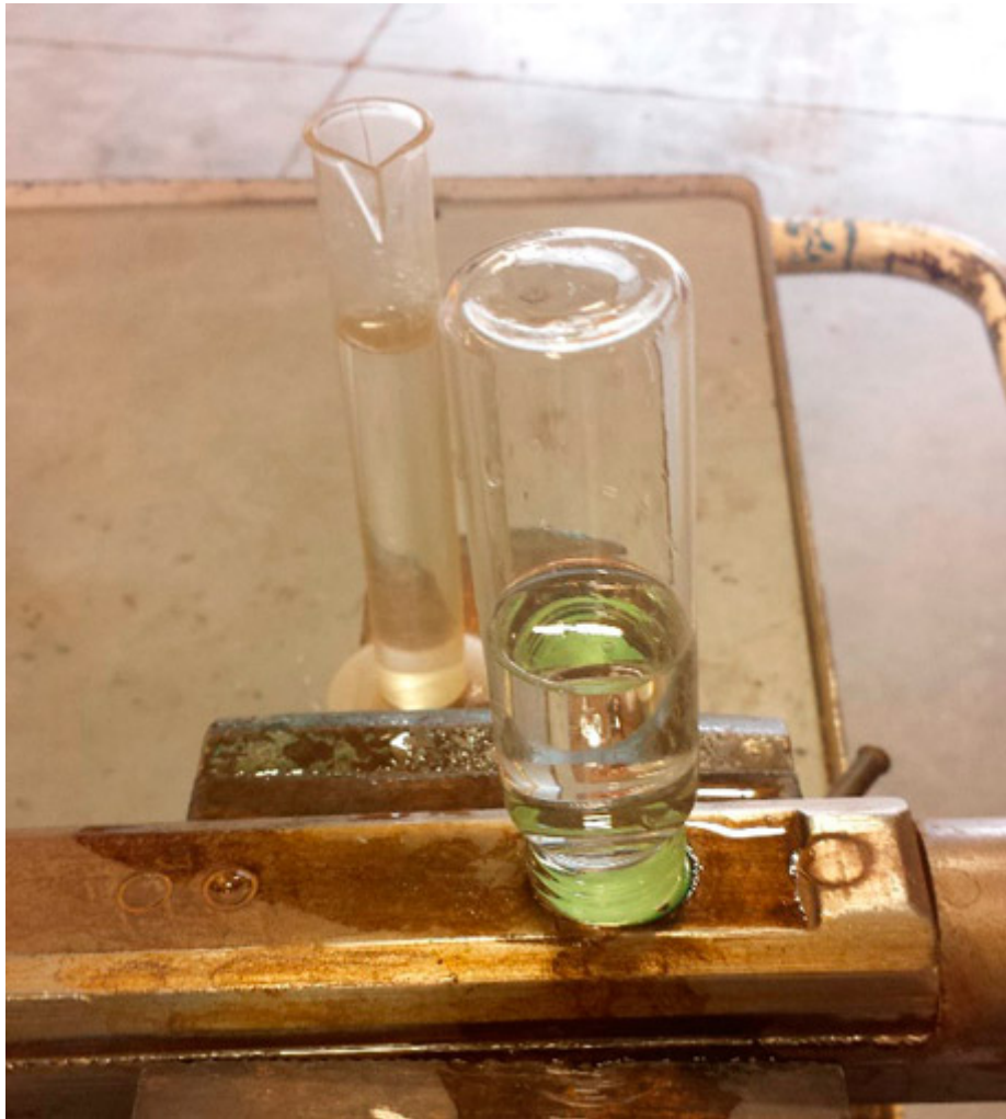
Figure 3-5. Response test - method of introducing an aqueous standard to the membrane.
