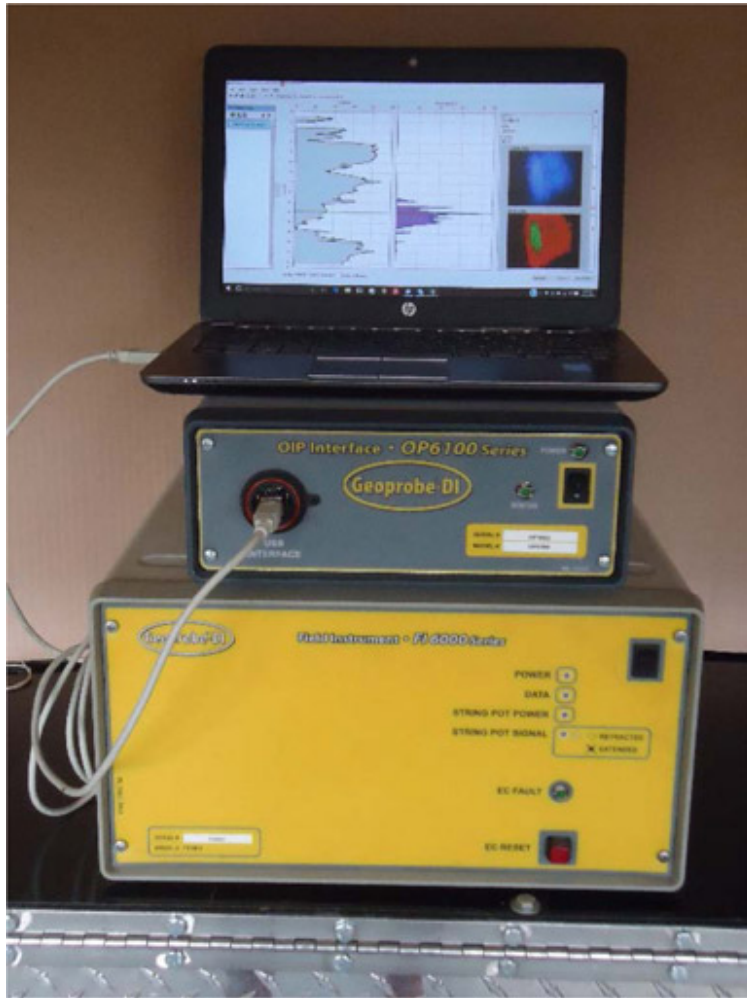
Figure 3-6. Aboveground OIP system components.
