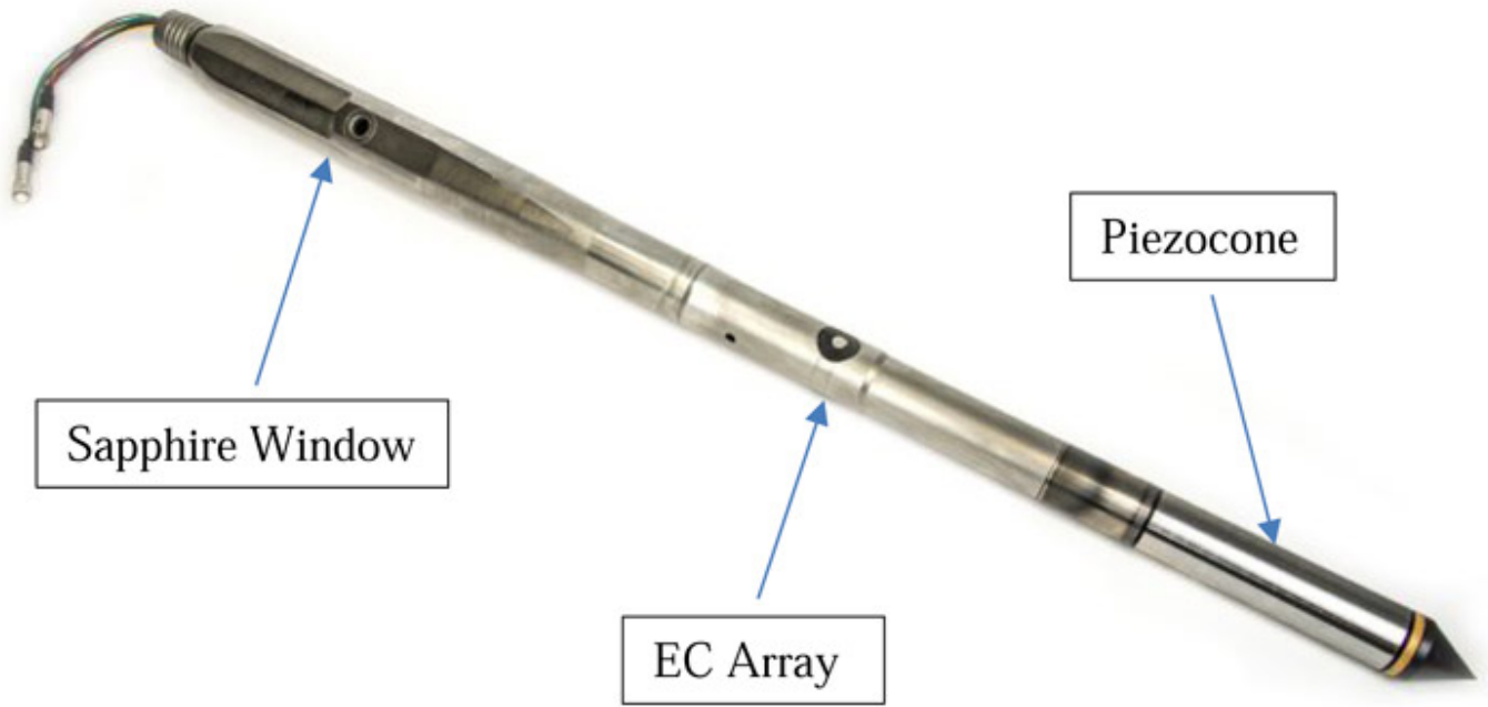
Figure 3-9. OIP probe with attached CPT cone.
