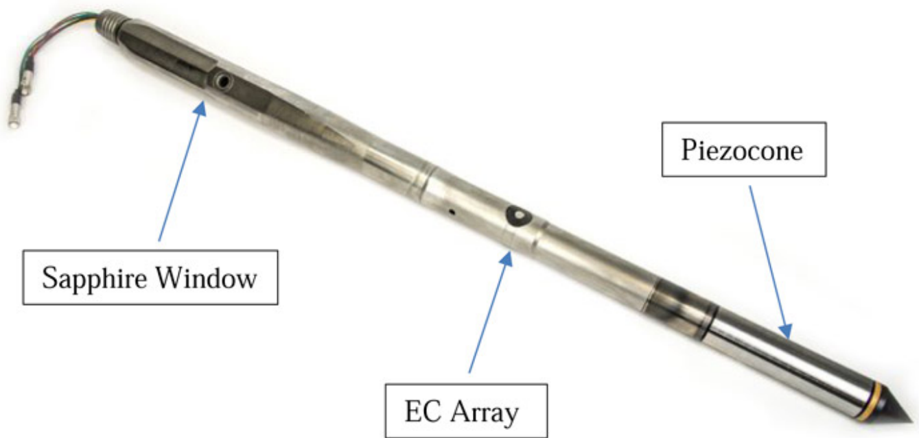
Figure 3-9. OIP probe with attached CPT cone.
