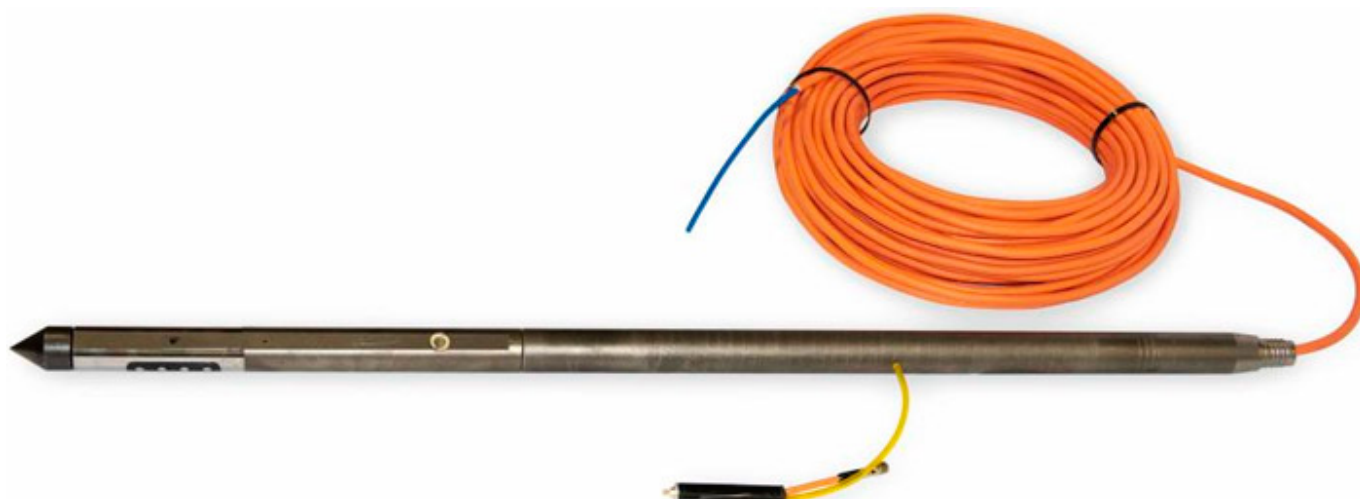
Figure 3-25. Downhole probe components of the HPT (The pressure sensor is shown outside of the connection rod but is actually located inside the rod during use).
