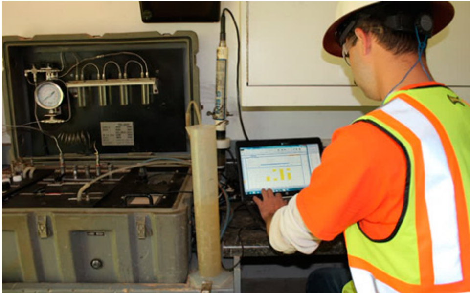
Figure 3-28. Waterloo APS operator purging groundwater from the sample interval, recording water-quality parameters, and preparing for sample collection.
