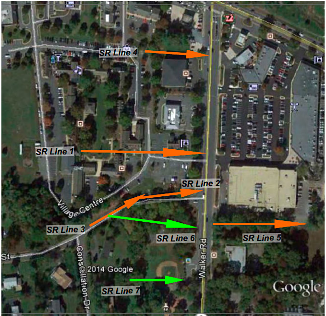
Figure 9-51. ER lines conducted on the site
