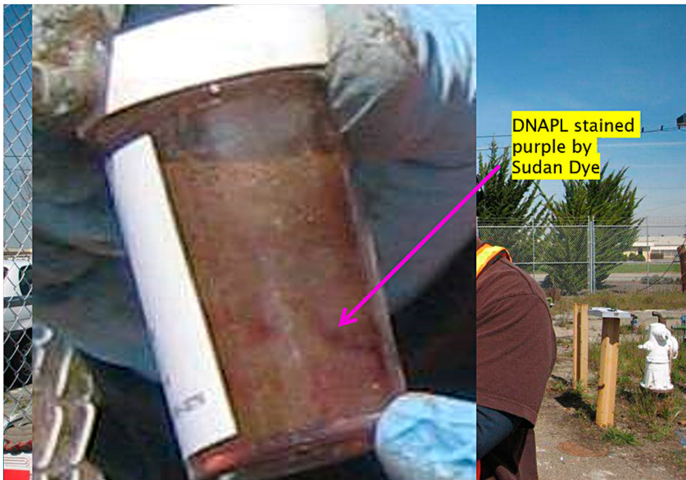
Figure 9-7. Sudan Dye staining indicating TCE DNAPL.
