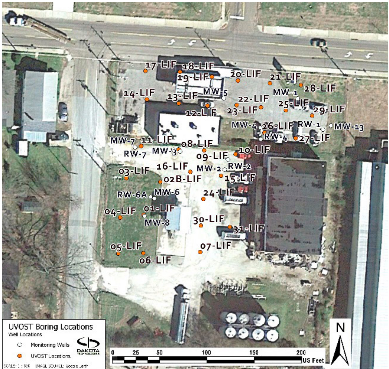
Figure 9-20. UVOST® boring and monitoring well locations.
